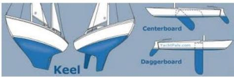
A diagram showing three types of keels: a traditional keel, a centerboard, and a daggerboard. The labels 'Keel', 'Centerboard', and 'Daggerboard' are included. | 主動控制      | 依風向被動控制  |
