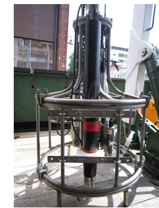
The turbulence package with CTD
