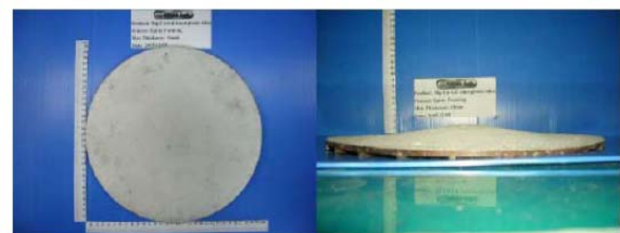
Fig. 4 Morphology of a spray-formed Mg-Cu-Gd layered composite plate with a Gaussian-shape, and 300 mm in diameter, 12 mm in maximum thickness, and 510 g in mass [40].
