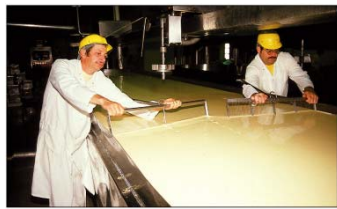
(a) The milk has been coagulated by the action of rennin (forming curd) and is inoculated with ripening bacteria for flavor and acidity. Here the workers are cutting the curd into slabs.
