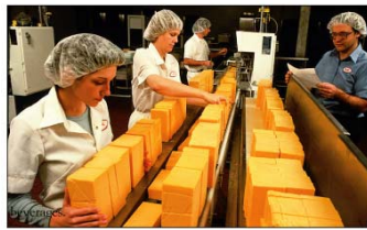
(c) The curd is milled to allow even more drainage of whey and is compressed into blocks for extended ripening. The longer the ripening period, the more acidic (sharper) the cheese.
